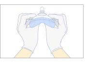
Put on the protective gloves. Unfold mask and check that filter is firmly in place.
